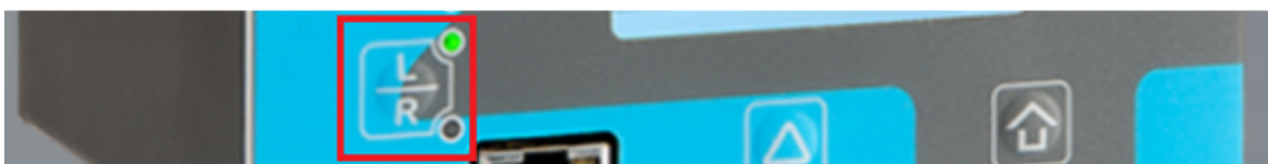
The Local/Remote switch at Local mode
